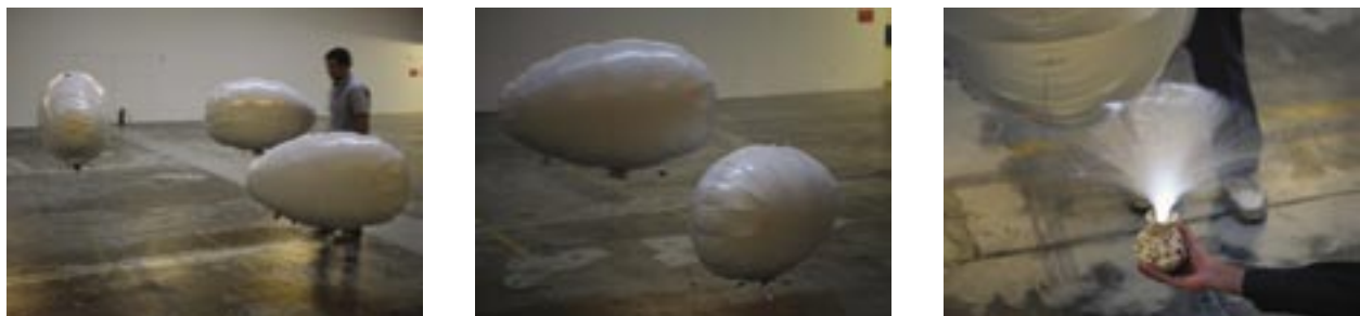
ALAVs are three flying objects that exist in a networked environment and communicate through assigned behaviors forming three scenarios: ALAVs alone: autonomous, ALAV with other ALAVs: flocking, and ALAVs with people: feeding. They are autonomous with respect to their decision making process and have an algorithm that defines how they roam in search of people or food (left). Within close proximity the ALAVs recognize another's presence and commence a flocking behavior. The behavior consists of ALAVs spinning together and calling back and fourth between each other (middle). The ALAVs interact with people by metaphorically feeding from a food device. If they are hungry they will respond when approached and begin a feeding behavior (right).
